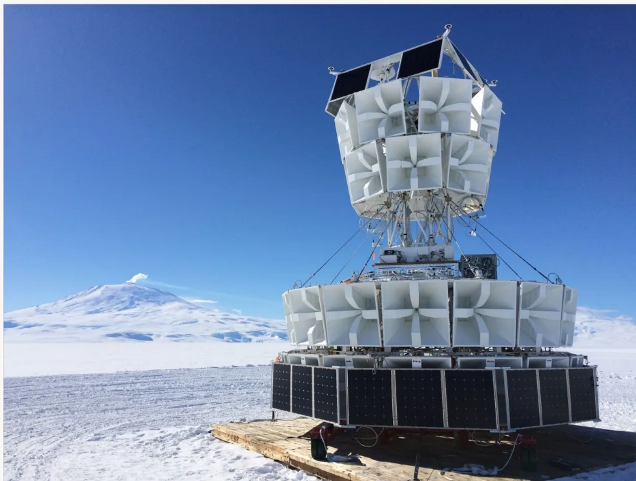
ANITA's 48 antennas are aimed down at the Antarctic ice on a 25-foot-tall gondola.
